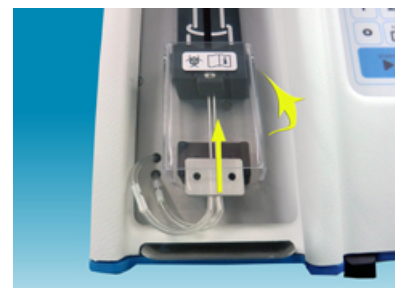
2. Place the needle sealing block into the needle guide block. Push the needle back upwards against the friction.
