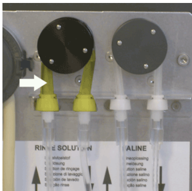
New rinse pump tube assembly ESRI090902.
