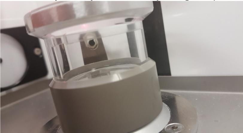
With the pO2 sensor spot removed and the cup sent to the home position, the fiber optic cable is visible through the sensor spot hole. This alignment is critical to accurately measure the pO2 sensor spot.
