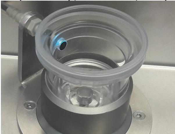
2. Replace the spot by a new one provided in a black plastic pouch by pressing it into the outside of the cup
