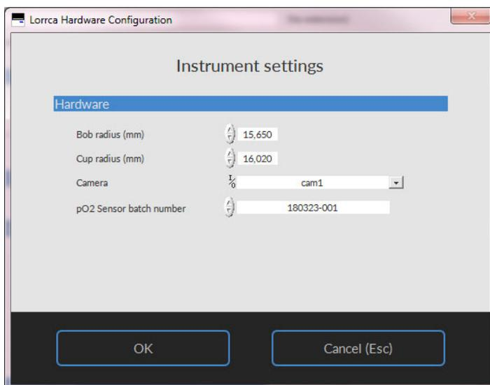
5. Select at **PO2 Sensor batch number** the correct calibration file, which is given with the sensor-spot. If the new calibration file cannot be found after replacement of the sensor-spot, the following warning is given
